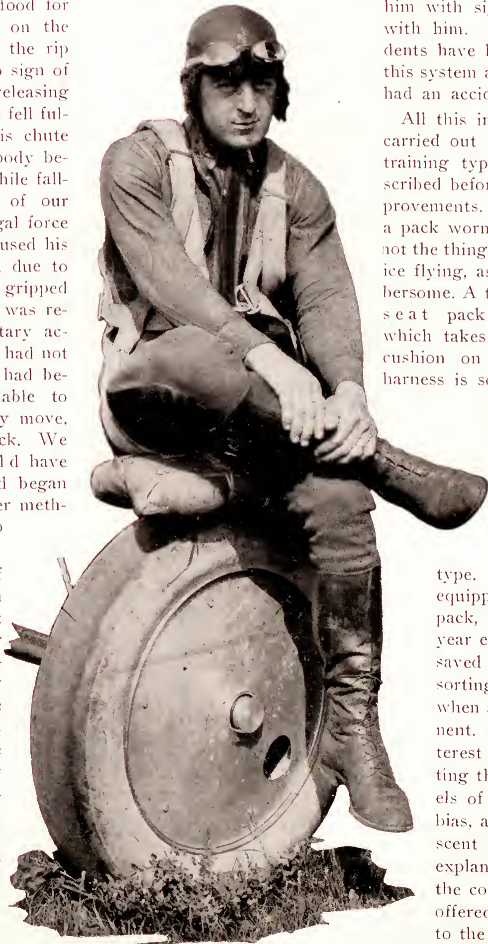
Showing the position of the seat type parachute pack now used as standard by all U. S. pilots.
